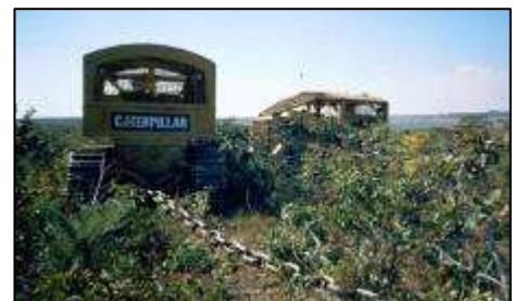
Deforestation of Cerrado by bulldozers pulling a steel chain in between them. © Ulrike Bickel
